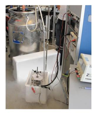
Figure 5. The HTS machine prototype setup after cool-down and during testing.
