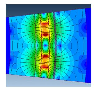
Figure 8. FE model of one pole pair of a 10MW HTS wind turbine generator set up and analysed by the second group.
